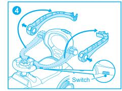
Push the switch of the armrest guardrail and spin it backward, the armrest guardrail can be removed.
