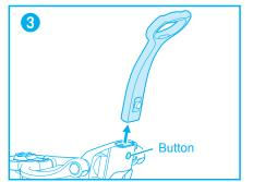
Press the button under the push knob, the push knob can be removed.
