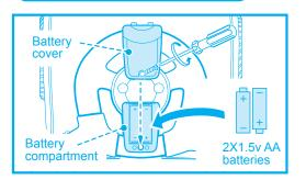
Open the steering wheel battery cover, find the positive pole and negative pole, and put 2AA batteries into the compartment properly, then close the battery cover and fix it with the screw (as shown in the Figure).
